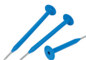
Insulation dowel SFS RP50/BS-4,8 wood (XFM 006) – distancer / fastener. Same product works as a fastener for the insulation as well as a distancer for 180-mm thick wind-protection insulation.
