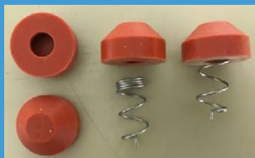
Option 2: Single spacers with springs recommended for pipes with \leq 30 mm diameter and smaller areas of insulation (e. g. inspection hatches) as well as pipe elbows
