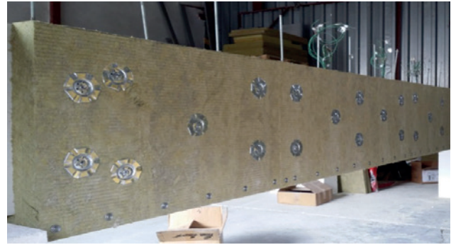
Fire protected concrete beam.
