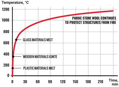
\* A "standard fire" simulates the development of temperatures in a fire in a normal room space according to the standard combustion curve ISO 834
