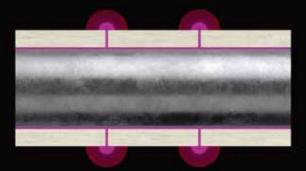
JOINTS IN STANDARD INSULATION WILL OPEN **DUE TO THERMAL EXPANSION OF THE PIPE WHEN HEATED**
