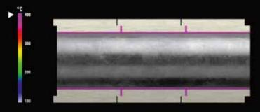
PAROC PRO LOCK'S Z-LOCK JOINTS WILL PREVENT THE SIGNIFICANT HEAT LOSS **CAUSED BY THERMAL EXPANSION OF THE HEATED PIPE**
